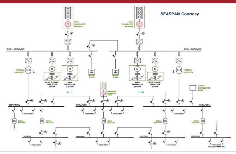
In addition to the LNG propulsion system the vessel will be fitted with a battery bank which an energy storage system (ESS). The vessels will use a 1050VDC, 546kWh ESS consisting of 84 Corvus Energy AT6500 advanced lithium polymer batteries. The ESS will be integrated with the electrical propulsion and distribution system and will be capable of providing power for propulsion for limited periods of time in lieu of the main engines.
